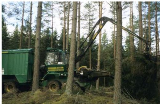
Figure 3.10. Collection and chipping of logging residues with a mobile chipper-forwarder Chipset 536C, photo by P. Muiste
