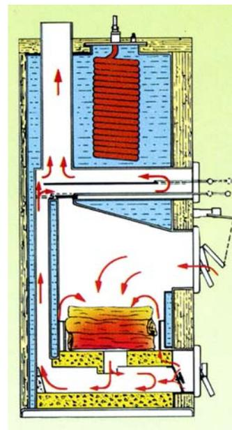
Figure 4.24. The reverse fired boiler EXONOM A25 BX MILJÖ made by the Swedish company EURONOM where a spiral heat exchanger is installed in the water volume
