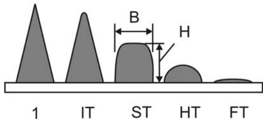
Figure 2.5. Fusibility characteristics of ash
