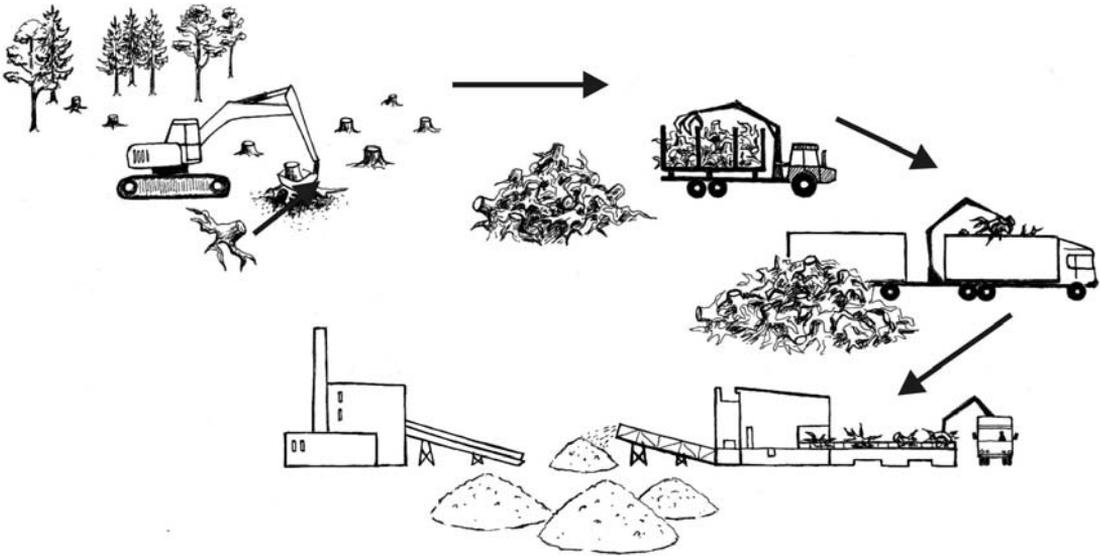
Figure 3.23. Stump rooting and haulage with a forwarder, transport with a special truck and crushing in the terminal
