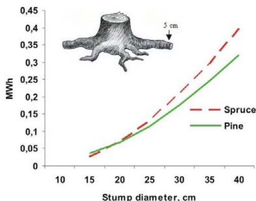
Figure 3.2. The heating value of stump-root system depending on the stump diameter [21]
