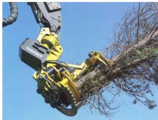
Figure 3.53. The accumulating shear heads Timberjack 720 and Timberjack 730 [35]
