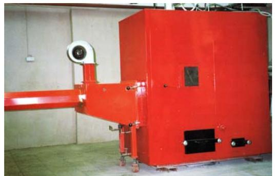
Figure 4.21. Solid fuel burner of Tallinn University of Technology with a 240 kW universal boiler
