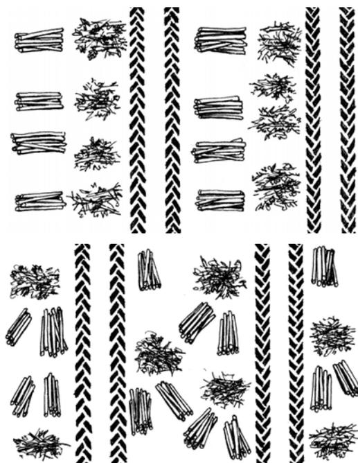
Figure 3.9. It is recommended to store delimbed branches separately during cutting operations
