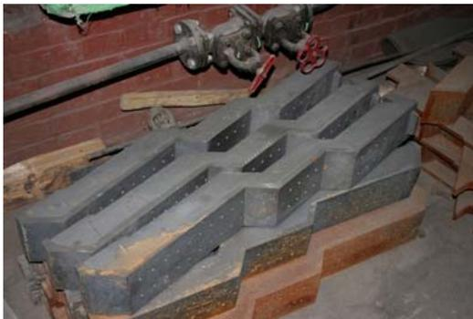
Figure 8.13. New grate bars of Tartu Foundry, photo by Ü. Kask
