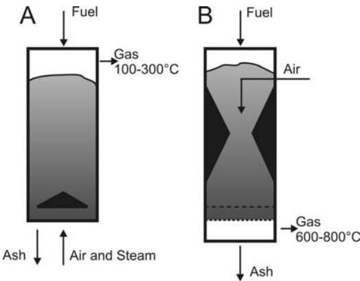
Figure 4.11. Schematic diagram of updraft (A) and downdraft (B) gasifiers
