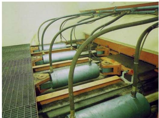
Figure 5.6. Hydraulic cylinders driving the push floor elements (Saxlund)
