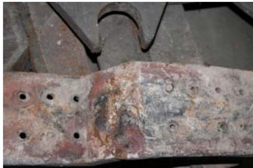
Figure 8.14. A grate bar after a year in the boiler, photo by Ü. Kask
