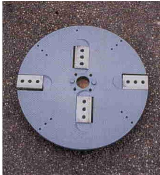
Figure 3.27. The operative part of a disc chipper, photo by P. Muiste
