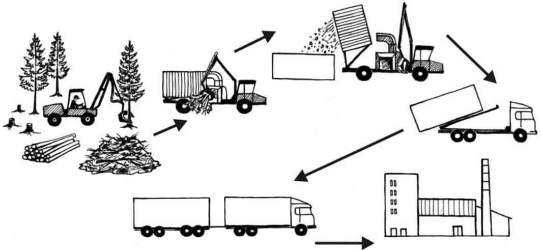
Figure 3.12. Haulage and chipping of logging residues in the cutting site with a mobile chipper-forwarder, transport with a woodchip trailer-truck
