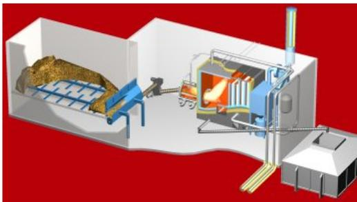
Figure 4.1. Layout of the equipment in a biofuel fired boiler plant, Thermia OY, Finland
