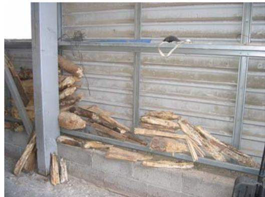
*Figure 8.35. Some examples of debris and uncrushed wood screened out from the fuel, photo by Ü. Kask*
