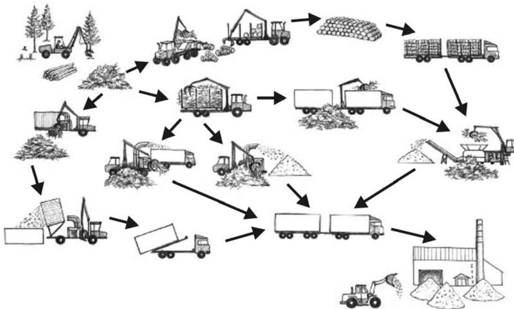
Figure 3.7. Production of woodchips from logging residues
