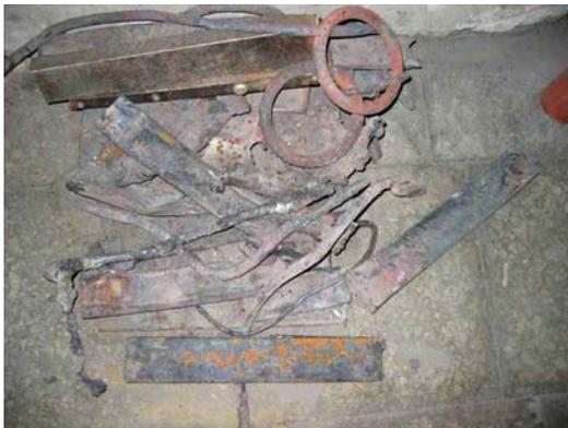
Figure 8.25. Some examples of metal pieces collected from fuel and ash, photo by Ü. Kask
