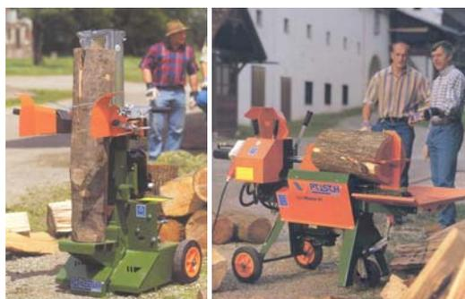
Figure 3.51. Choppers with a hydraulic drive [39]
