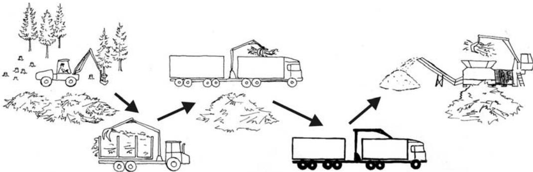
Figure 3.21. Transport with a trailer-truck
