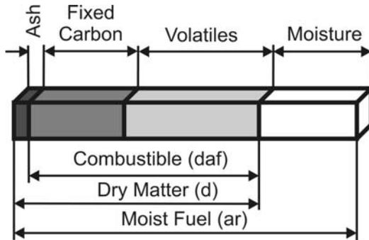
Figure 2.3. Components of solid fuel
