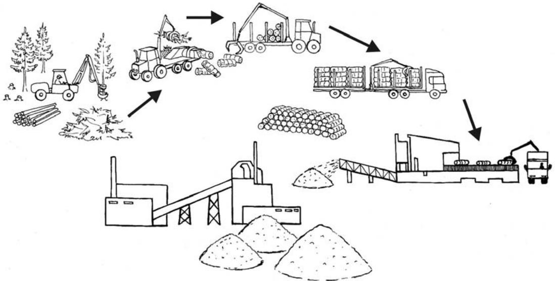
*Figure 3.22. Baling of logging residues, haulage with traditional forwarders and logging trucks, chipping in the terminal*
