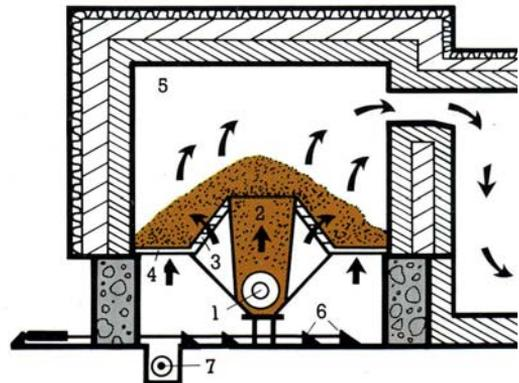
Figure 4.3. Underfed pre-furnace with a conical grate (retort grate) for burning very wet fuel, SERMET, Finland
