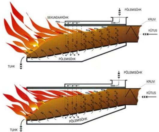
Figure 4.20. Burner layouts for dry (upper) and moist (lower) fuels developed at Tallinn University of Technology
