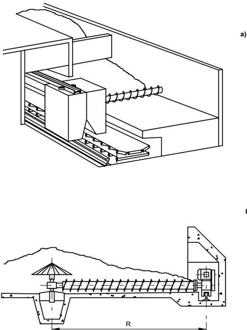
Figure 5.8. Screw conveyors in the bunker bottom
