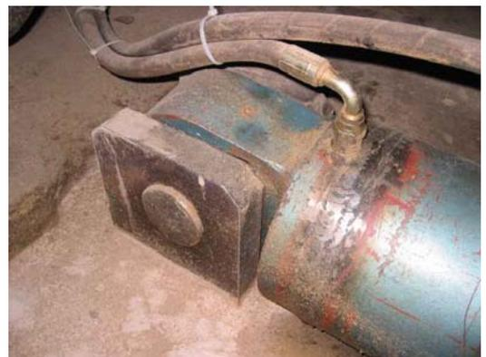
*Figure 8.29. Welded ending part of hydraulic cylinder, photo Ü. Kask*
