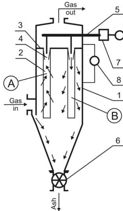
Figure 6.2. Bag filter with pulse jet cleaning
