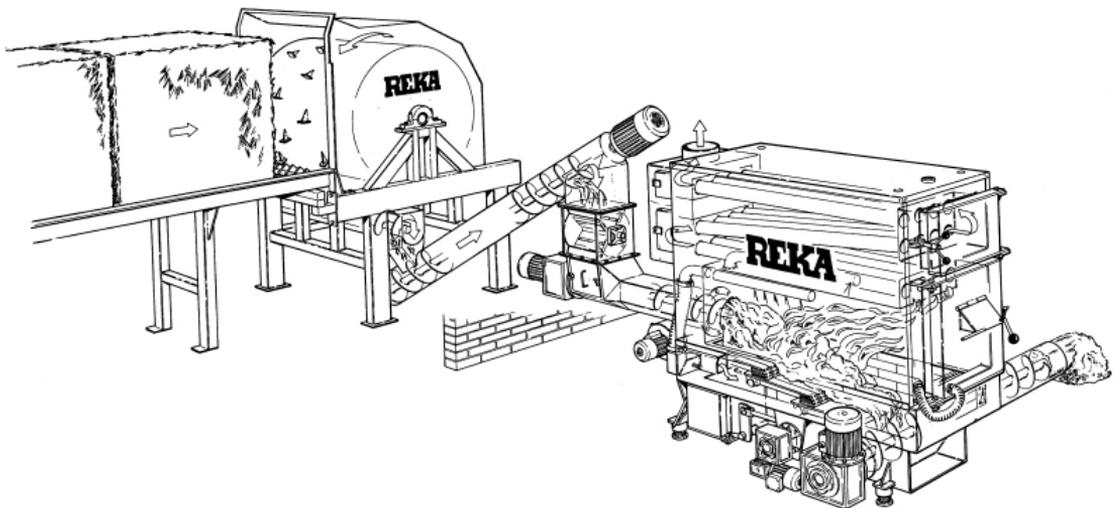
Figure 4.15. Automatic straw combustion system with the straw bale shredding unit [44]
