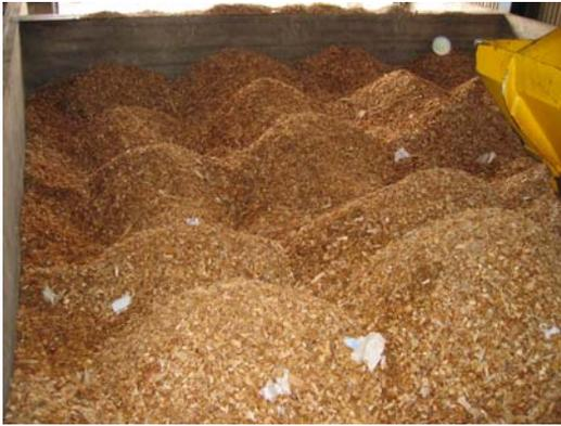
*Figure 8.10. Computer controlled grab crane has distributed fuel uniformly over the storage area, photo by Ü. Kask*
