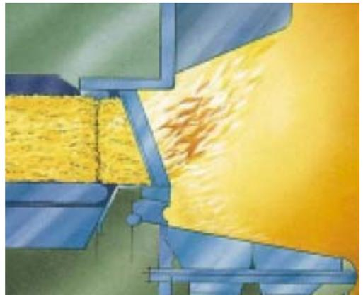
Figure 4.14. „Cigar-type” combustion method with the successive feeding of straw bales [44]
