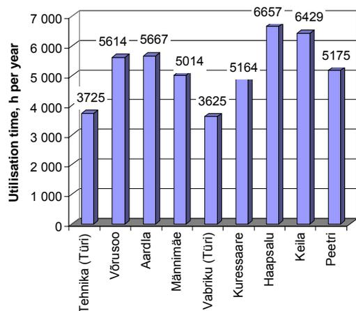
Figure 8.44. Calculated utilisation time of biofuel boilers in 2004
