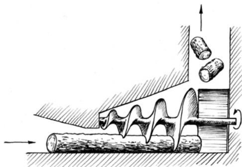
Figure 3.30. A screw chipper
