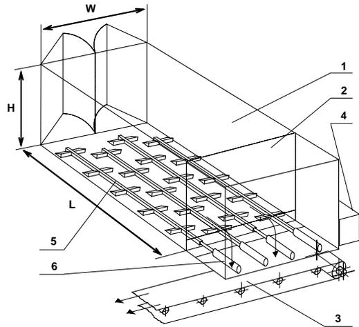
Figure 5.5. Solid fuel bunker with pushers
