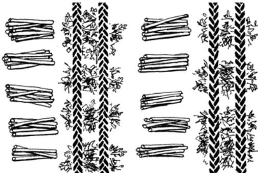
Figure 3.8. Use of logging residues for branch mats on the haulage roadways [24]
