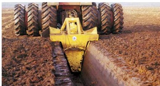
*Figure 3.65. Pressing of drainage ditches in the bog soil with the ditcher OJ-1.3K made by the Finnish SUOKONE OY*
