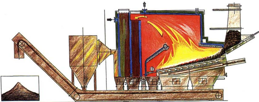
Figure 4.7. The integrated PMA type boiler plant for solid fuels of Finnish company Putkimaa OY with the capacity range of 1 – 10 MW
