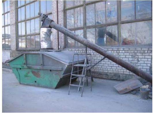
A. Ash container with a screw conveyor
