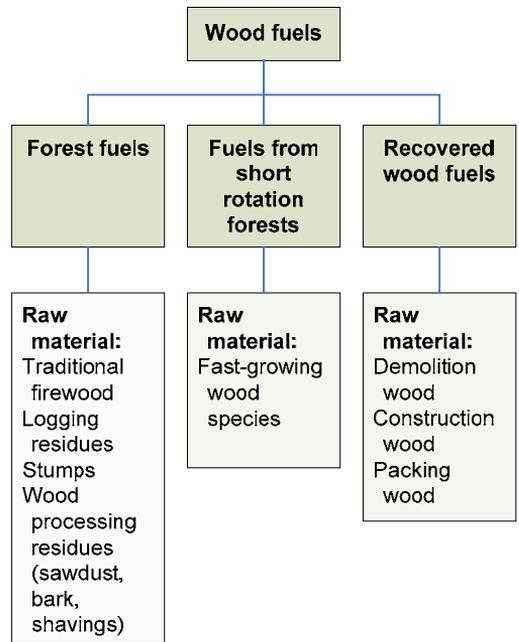
Figure 2.1. Wood fuel classification based on the origin of raw material
