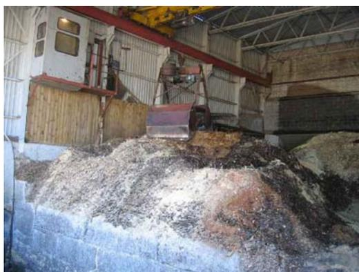
*Figure 8.32. Manned bridge crane with grabber, photo by Ü. Kask*
