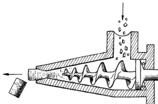
Figure 3.55. A screw extruder
