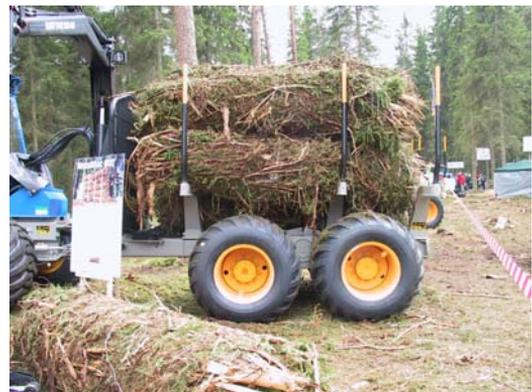
Figure 3.48. A simple logging truck-trailer can be used for the transport of baled logging residues, photo by P. Muiste
