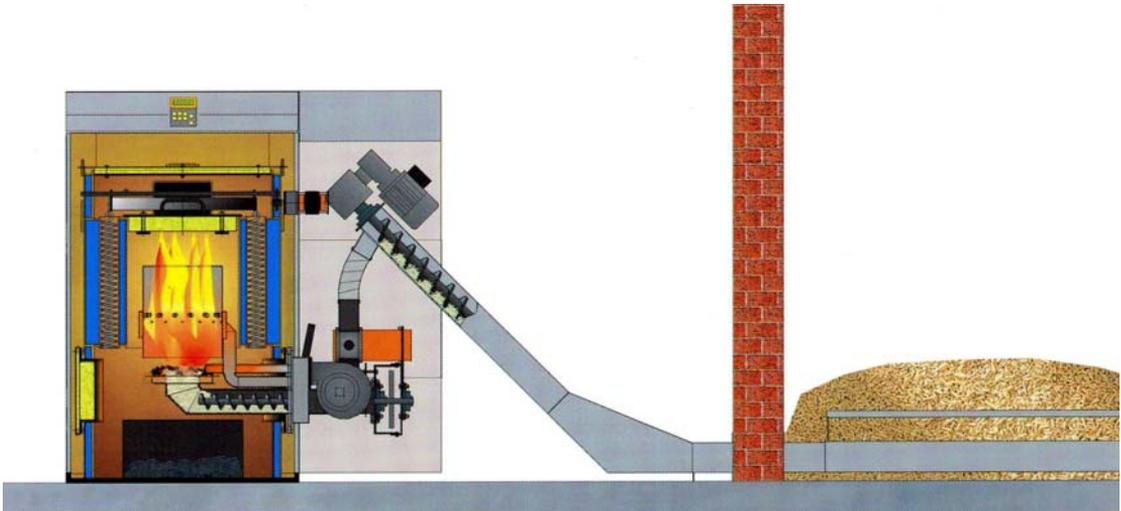
Figure 4.16. Principle scheme of the pellet combustion system [56]
