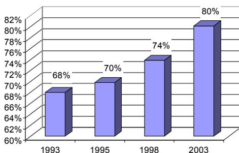
*Figure 8.4. The average annual efficiency of wood and peat fired boilers according to statistics*
