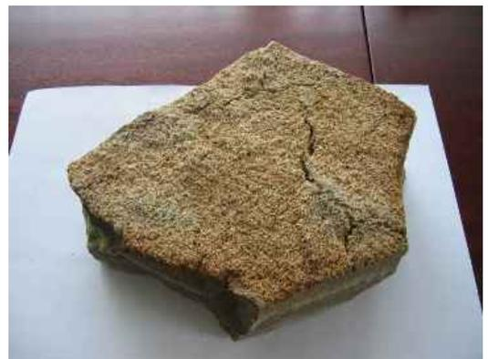
*Figure 8.40. A piece of deposit removed from the furnace, photo by Ü. Kask*
