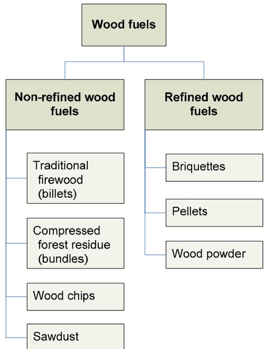
Figure 2.2. Wood fuel classification based on the upgrading level
