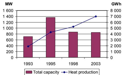
Figure 8.2. Development of total capacity and heat production of the wood and peat fired boilers
