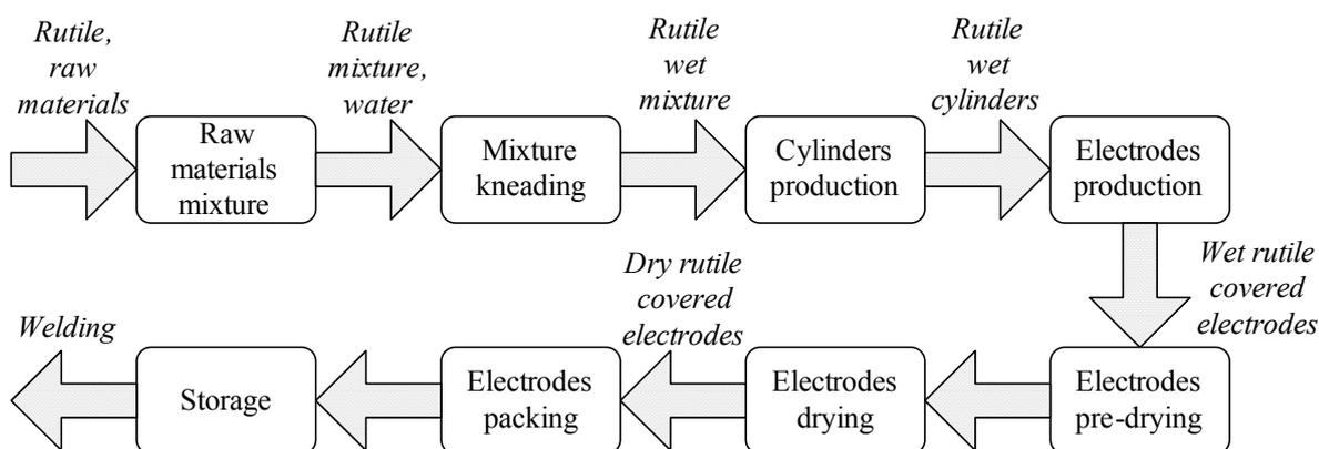
**Figure 1. Process of rutile covered electrodes manufacturing.**
