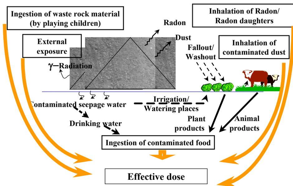
**Figure 1. Exposure pathways for members of the local public living next to an uncover-red radioactive waste rock pile**
