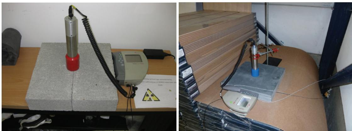
**Figure 1. B-NORM method: counting a sample**
