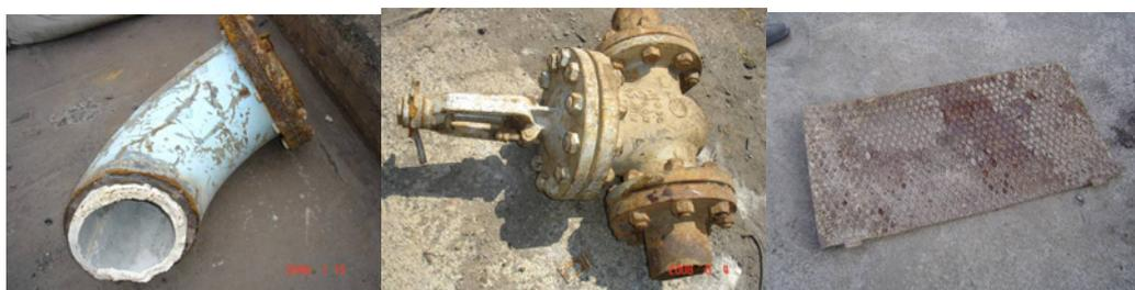
**Figure 2. Typical pieces contaminated with Norm (sheet, pipe, valve)**
