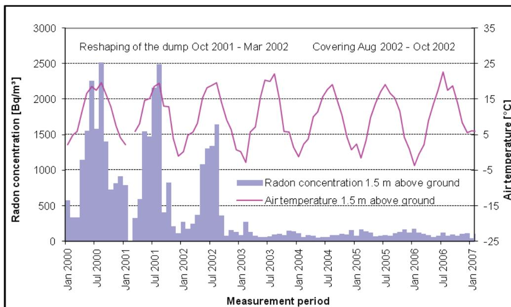
**Figure 5. Evolution of pre- and post-rehabilitation radon concentrations at the mine dump 66/207, Wismut site Alberoda**
