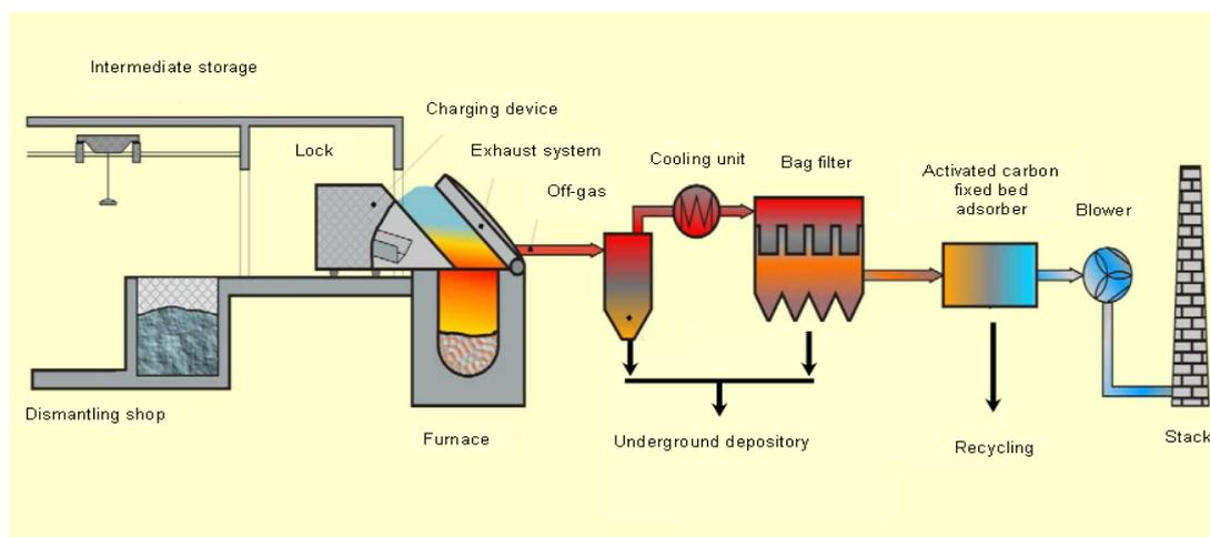
**Figure 1. Layout of GERTA Melting plant**
