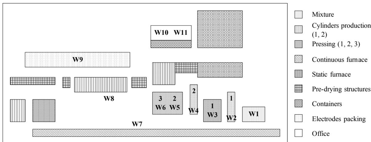
**Figure 2. Covered electrodes production area diagram and workers positions.**
