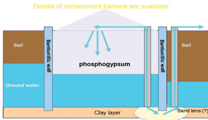
**Figure 1: Schematic view of the Gela PG stack**
