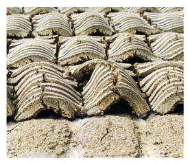
Figure 3.67. The wave-like extruded sod peat that provides minimum contact with the bog surface and therefore dries faster
