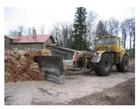
Figure 8.31. Tractor adapted for fuel moving, photo by Ü. Kask
