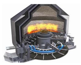
Figure 4.6. The Wärtsilä patented BioGrate furnace with an underfed rotating conical grate
