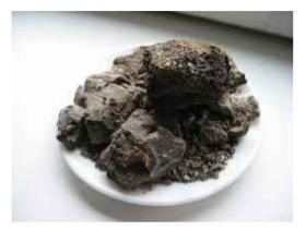
Figure 8.8. Hardened ash deposits from the curved arch, photo by Ü. Kask
