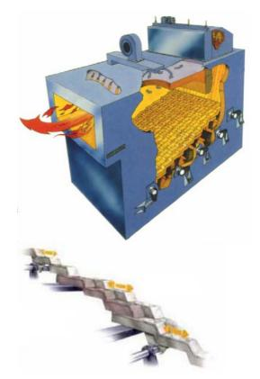
Figure 4.5. The Swedish KMW ENERGI AB TRF furnace with checkered grate bars
