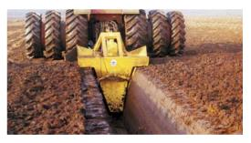
Figure 3.65. Pressing of drainage ditches in the bog soil with the ditcher OJ-1.3K made by the Finnish SUOKONE OY
