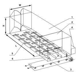
Figure 5.5. Solid fuel bunker with pushers
