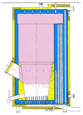
Figure 4.10. The PML type fluidized bed gas tube boiler of the 1 – 5 MW capacity (Putkimaa OY, Finland)
