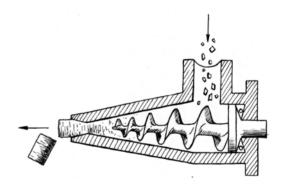
Figure 3.55. A screw extruder
