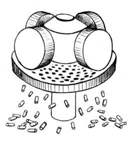
Figure 3.57. Pelletizer with flat die
