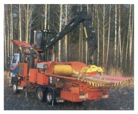
Figure 3.41. A chipper mounted on the Giant truck [32]
