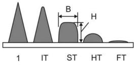
Figure 2.5. Fusibility characteristics of ash
