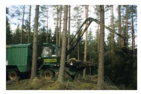
Figure 3.10. Collection and chipping of logging residues with a mobile chipper-forwarder Chipset 536C, photo by P. Muiste
