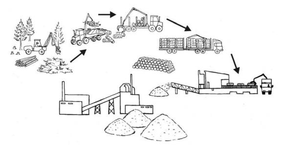
Figure 3.22. Baling of logging residues, haulage with traditional forwarders and logging trucks, chipping in the terminal
