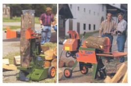
Figure 3.51. Choppers with a hydraulic drive [39]
