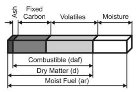
Figure 2.3. Components of solid fuel
