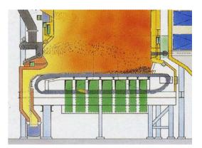
Figure 4.8. Travelling (chain) grate in the boiler of the Borås CHP plant (Sweden)
