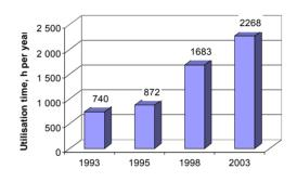
Figure 8.3. Change of the annual utilisation time of wood and peat fired boilers
