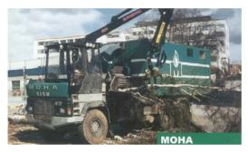
Figure 3.42. The Moha trailer-truck equipped with a chipper [32]
