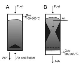
Figure 4.11. Schematic diagram of updraft (A) and downdraft (B) gasifiers
