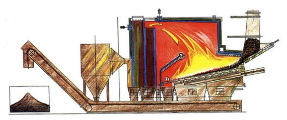
Figure 4.7. The integrated PMA type boiler plant for solid fuels of Finnish company Putkimaa OY with the capacity range of 1 - 10 MW
