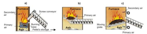
Figure 4.17. Technological solutions for the pellet feeding and combustion systems
