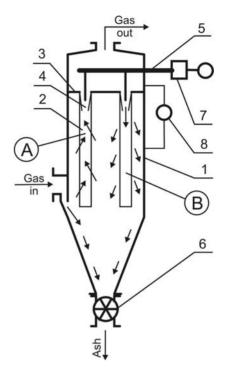
Figure 6.2. Bag filter with pulse jet cleaning
