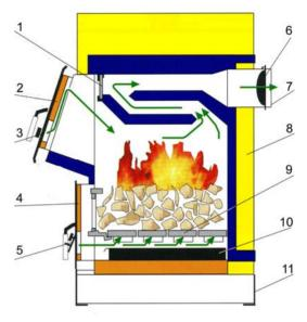
Figure 4.22. A top fired boiler from Eder Ltd (Austria)
