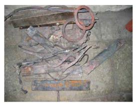
Figure 8.25. Some examples of metal pieces collected from fuel and ash, photo by Ü. Kask
