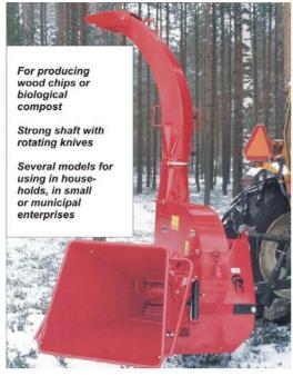
Figure 3.34. A disc chipper driven from the power take-off shaft of an agricultural tractor Junkkari HJ 10 [28]
