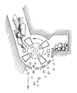
Figure 3.31. A hammer mill
