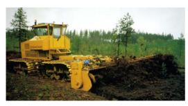
Figure 3.64. Vegetation stripping and levelling of peat bog surface with the screw leveller RT-6.0H made by the Finnish SUOKONE OY
