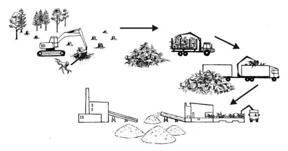
Figure 3.23. Stump rooting and haulage with a forwarder, transport with a special truck and crushing in the terminal
