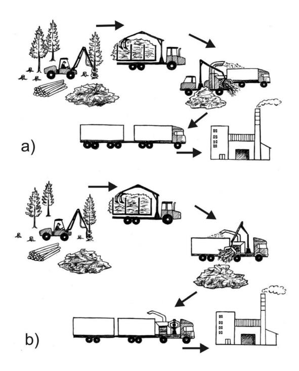
Figure 3.14. Roadside chipping of logging residues
