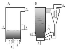
Figure 4.9. Schematic diagram of furnaces with bubbling (A) and circulating (B) fluidized beds
