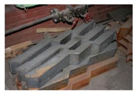
Figure 8.13. New grate bars of Tartu Foundry, photo by Ü. Kask
