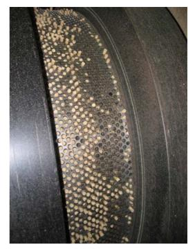
Figure 3.58. The cylindrical matrix of pelletizer, photo by P. Muiste
