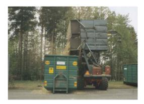
Figure 3.11. Dumping of the container of mobile chipper, photo by P. Muiste
