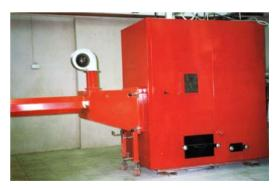
Figure 4.21. Solid fuel burner of Tallinn University of Technology with a 240 kW universal boiler
