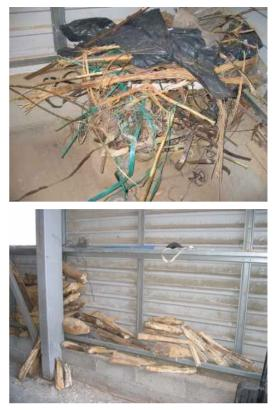
Figure 8.35. Some examples of debris and uncrushed wood screened out from the fuel, photo by Ü. Kask
