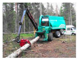
Figure 3.36. A mobile chipper-forwarder, Silvatec 878 CH [29], photo by P. Muiste
