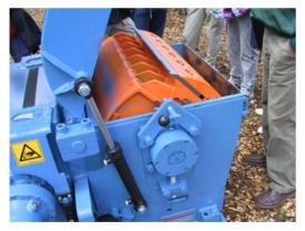
Figure 3.29. The operative part of a drum chipper, photo by P. Muiste
