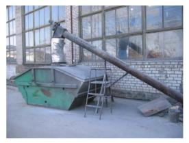
A. Ash container with a screw conveyor
