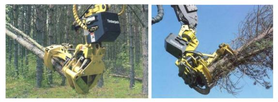
Figure 3.53. The accumulating shear heads Timberjack 720 and Timberjack 730 [35]
