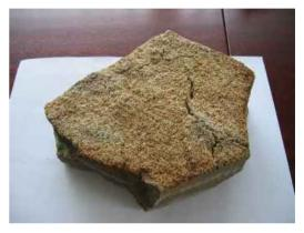
Figure 8.40. A piece of deposit removed from the furnace, photo by Ü. Kask
