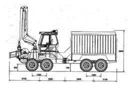
Figure 3.37. A mobile chipper-forwarder Chipset 536 C [30]
