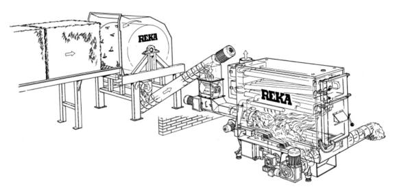
Figure 4.15. Automatic straw combustion system with the straw bale shredding unit [44]
