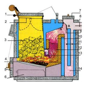
Figure 4.23. The Arimax bottom fired boiler, Högfors Lämpö OY, Finland
