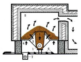
Figure 4.3. Underfed pre-furnace with a conical grate (retort grate) for burning very wet fuel, SERMET, Finland
