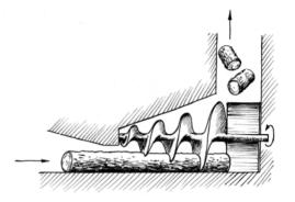
Figure 3.30. A screw chipper
