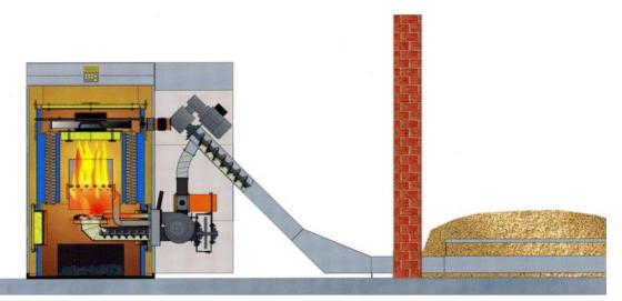
Figure 4.16. Principle scheme of the pellet combustion system [56]
