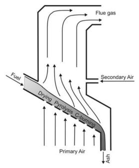
Figure 4.2. Combustion zones of moist biofuel on the sloping grate
