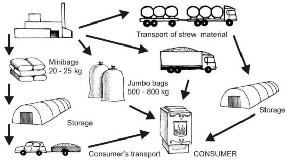
Figure 3.59. The pellet supply diagram
