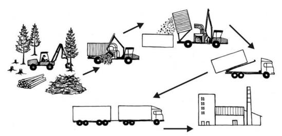
Figure 3.12. Haulage and chipping of logging residues in the cutting site with a mobile chipper-forwarder, transport with a woodchip trailer-truck
