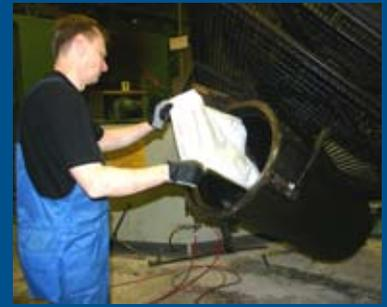
The thermoplastic raw material, a powder, is loaded into the moulds...
