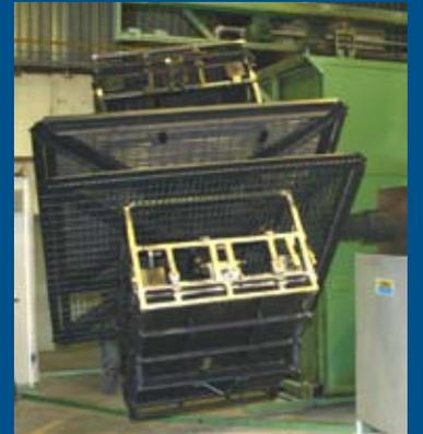
...under constant double rotation the moulds goes to the oven, heated up to 230° -240° C...
