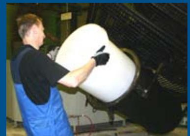
...after a production cycle that typically lasts for one hour, the products can be unloaded from the moulds...
