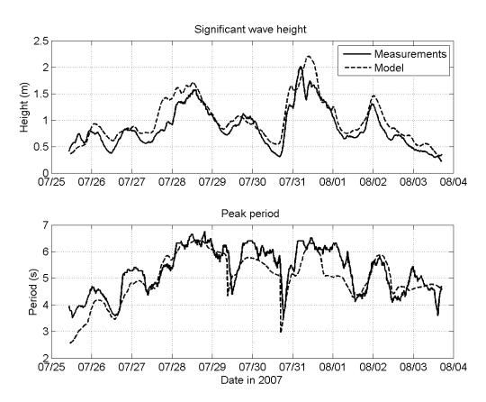
Figure 3 Model-data comparison at the location of the wind farm 2.
