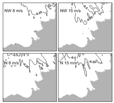
**Figure 6** The impact of the wind farm 2. The contour unit is [%] and a negative value shows a decrease of significant wave height.
