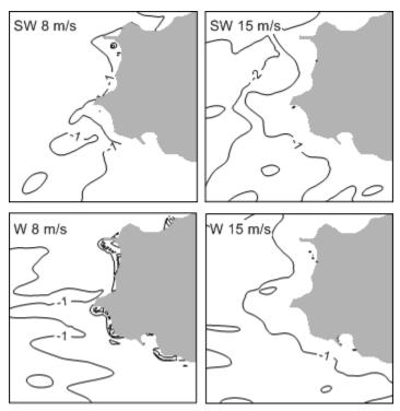
**Figure 5** The impact of the wind farm 1. The contour unit is [%] and a negative value shows a decrease of significant wave height.
