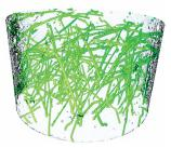
Fibre reinforced concrete and the 3D visualization of fibres
