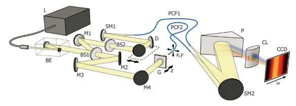
Interferometric set-up (acronym OCEAN TADPOLE)
