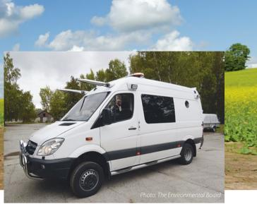
The Radiation Department of the EIC received a modern mobile laboratory that significantly increases Estonia's ability to react in emergencies, and perform environmental supervision and monitoring tasks.
