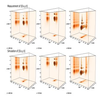
Figure 28: Measured (top) and simulated (bottom) impulse response of type IV Airy pulse generator consisting of a custom-made continuous cubic phase element and a Fourier lens f = 500mm at three propagation distances. Color represents the relative amplitude of the electric field isosurfaces. The images show projections of the pulse to the corresponding planes.
