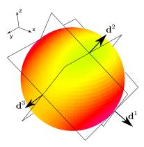
Figure 10: Orientation distribution of fibres with symmetry planes calculated from the second-order alignment tensor (eigenvectors are shown as well).
