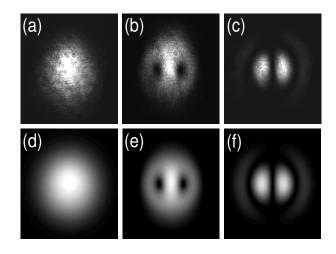
Figure 29: Experimental (top row) and theoretical (bottom row) profiles of the beams produced by conical refraction of a linearly polarized Gaussian input: without polarization selection (a, d); selected in parallel polarization (b,e); selected in orthogonal polarization (c, f). Each picture size is  $16 \times 16mm^2$ .
