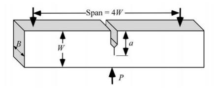
Figure 4: The general proportions of the specimen configuration.
