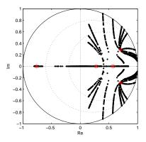
Figure 25: Root loci of the reflection segments bunch with the optimal controller.
