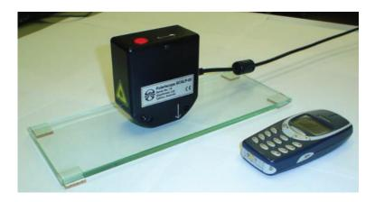
Figure 22: Scattered light polariscope SCALP for stress measurement in architectural glass panels and automotive glazing.
