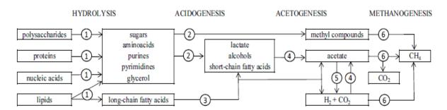
**Figure 1.** Stages of anaerobic digestion of the organic matter: 1) hydrolysis of biopolymers, 2) acidogenesis, 3) β-oxidation of long-chain fatty acids, 4) acetogenesis, 5) acetate oxidation, 6) methanogenesis. Modified from Insam et al (2010).
