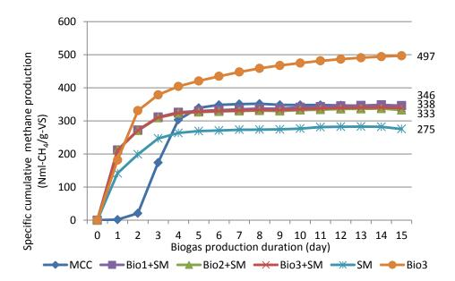
**Figure 6.** Specific cumulative methane production of different experimental lines in AMPTS II. Experimental lines include MCC (positive control with microcrystalline cellulose); SM (sludge mixture of primary and excess sludge); Bio3 (food waste from third sampling); Bio1+SM, Bio2+SM, Bio3+SM (mixtures of different food waste samples and sludge mixture).
