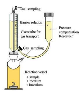
**A2.** Reaction system with eudiometer unit. The main parts of the eudiometer unit include the reaction vessel, the gas collection tube with barrier solution and a reservoir tank (Guwy 2004, modified from ISO/DIS14853 1999).
