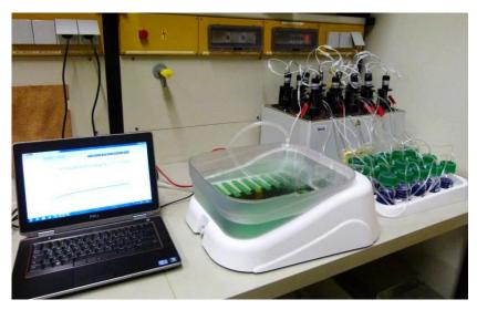
**A3.** AMPTS II instrument. The reactors in a white water bath are situated in the back right of the image; in the front right CO<sub>2</sub> trap bottles can be seen; the white device in the middle is methane detection unit, which sends online data to the computer.
