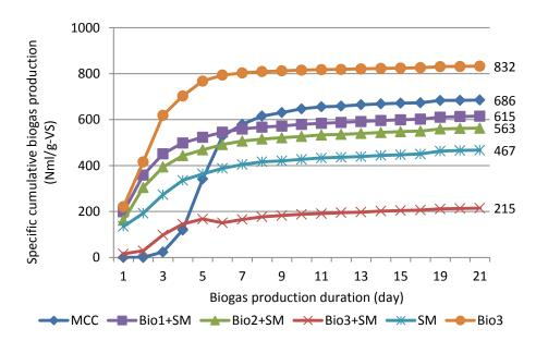
**Figure 5.** Specific cumulative biogas production of different experimental lines in liquid displacement system. Experimental lines include MCC (positive control with microcrystalline cellulose); SM (sludge mixture of primary and excess sludge); Bio3 (food waste from third sampling); Bio1+SM, Bio2+SM, Bio3+SM (mixtures of different food waste samples and sludge mixture).
