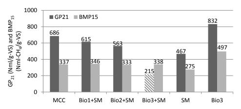
**Figure 7.** Biogas potential GP<sub>21</sub> and biological methane potential BMP<sub>15</sub> of the experimental lines. Experimental lines include MCC (positive control with microcrystalline cellulose); SM (sludge mixture of primary and excess sludge); Bio3 (food waste from third sampling); Bio1+SM, Bio2+SM, Bio3+SM (mixtures of different food waste samples and sludge mixture). GP<sub>21</sub> of Bio3+SM (hatched diagonally) should not be validated due to a technical error in the experiment.
