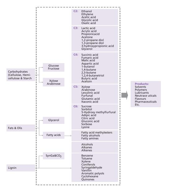
Figure 7: Chemicals and products that can be obtained through biochemical processing of biomass
