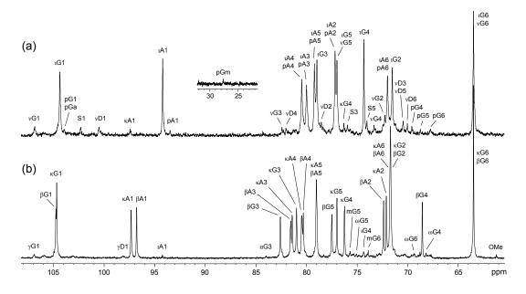
**Figure 7.** <sup>13</sup>C-NMR spectra of water-extracted galactans from the Kassari algal community. (a) Galactans from *C. truncatus*, 38,000 transients, recorded at 40 °C; (b) galactans from *F. lumbricalis*, 100,000 transients, recorded at 50 °C. S – glucose units in floridean starch. For other signal marks and chemical shift values, see Figure 8.
