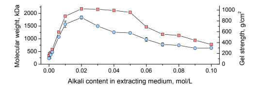
**Figure 13.** Dependence of furcellaran (**•**) gel strength and (**•**) molecular weight characteristic on KOH content in the extracting medium.
