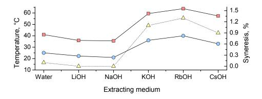
**Figure 14.** Characteristics of 1.5% furcellaran gels in the presence of different counterions. Galactans extracted 4 hours in 0.02 M alkali metal hydroxide solutions or in pure water. (**a**) Gel melting temperature; (**o**) gelling temperature; ( $\Delta$ ) syneresis value.
