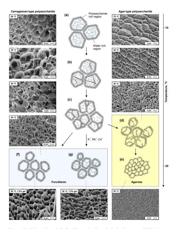
**Figure 12.** Schematic model of gel formation for red algal galactans and SEM images of cryofixated gelling states (upon cooling) of 2% water-extracted furcellaran and agarose (Serva) preparations. Micrograph of cation-mediated gel structure represents 1.5% water-extracted furcellaran gelled in 0.01 M RbCl solution. For letter mark meanings see the text.
