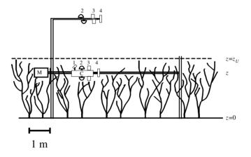
**Figure 4.1:** Radiation measurement system inside the willow coppice. M - drive, C – carriage, 1 – sunfleck indicator, 2 – pyranometer, 3 – quantum PAR sensor, 4 – net radiometer.
