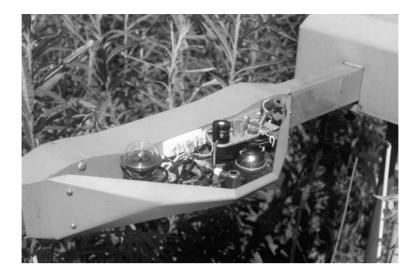
Figure 4.2: Photo of the sensor carriage inside the S. viminalis coppice.
