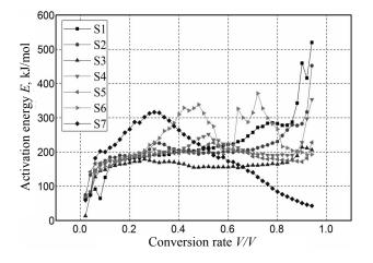
Fig. 3. Activation energies for samples S1 to S7 as a function of conversion rate.
