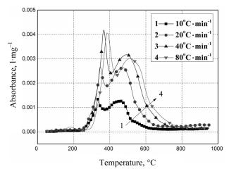
Fig. 5. Gram-Schmidt curves for the combustion of sample S3 at different heating rates.
