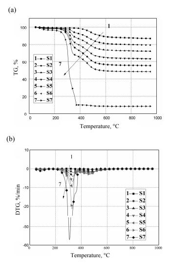
Fig. 1. (a) Thermogravimetric (TG) and (b) derivative thermogravimetric (DTG) combustion curves for samples S1 to S7 at a heating rate of 20  $^{\circ}$ C/min.
