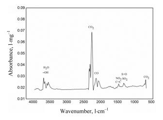
Fig. 7. FTIR spectrogram for the combustion of sample S3 at 472.62  $^{\circ}\mathrm{C}$
