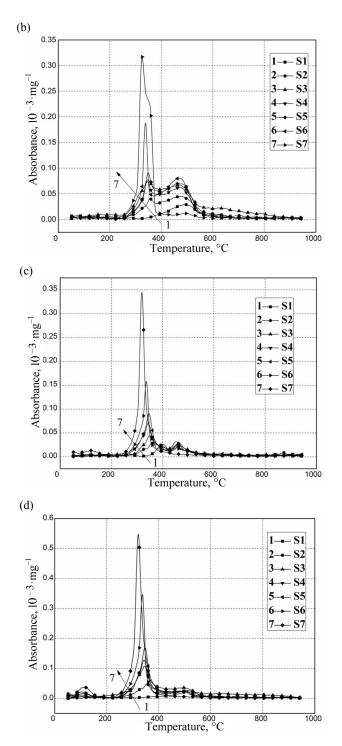
Fig. 8. FTIR absorbance curves for some specific gaseous products during the combustion of samples S1 to S7: (a)  $CO_2$  (2306 cm<sup>-1</sup>); (b) CO (2182 cm<sup>-1</sup>); (c) SO<sub>2</sub> (1374 cm<sup>-1</sup>); (d) NO<sub>2</sub> (1510 cm<sup>-1</sup>).
