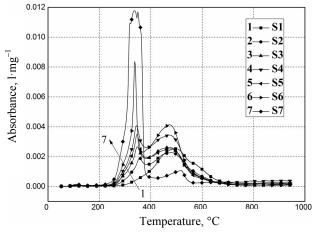
Fig. 4. Gram-Schmidt curves for the combustion of samples S1 to S7 at a heating rate of 20  $^{\circ}$ C/min.
