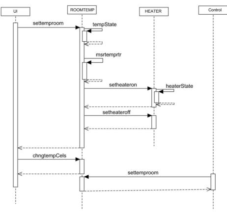
Fig. 4. Sequence diagram for temperature control of the e-home system.
