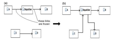
Fig. 3. Freezing dispatcher connection: (a) before genetic architecture synthesis, (b) after genetic architecture synthesis.
