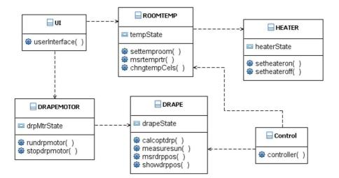
Fig. 5. Null architecture for the e-home system.
