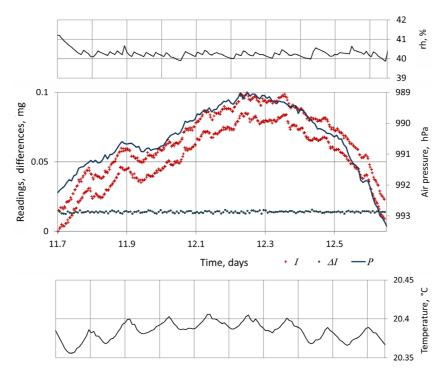
Fig. 1. One-day measurement sequence: readings (+) and mass differences (•). Solid lines show relative humidity (rh), air pressure, and temperature inside the comparator chamber.
