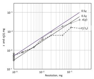
Fig. 5. Standard deviation and the Allan deviation as a function of digital resolution q. Straight lines show the range from 0.3q to 0.5q of the respective resolution.
