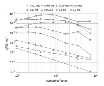
**Fig. 3.** Allan variance of measured mass differences as a function of averaging factor m and digital resolution q.
