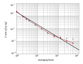
**Fig. 2.** Determination of the lowest limit for uncertainty from the  $\sigma^2 - \tau$  plot. The Allan variance is shown with squares,  $s^2$  with open circles, and both together with the expanded uncertainty interval; k = 2. The white noise 1/n dependence of variance is shown as a straight line.
