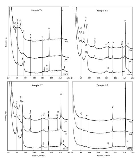
Fig. 5. X-ray diffraction analyses of the < 2  $\mu$  fraction of the four studied samples: Nat – untreated sample; EG – glycolated sample; H – sample heated to 550 °C; Ch – chlorite; IS – interstratified illite and smectite; I – illite; K – kaolinite; Q – quartz; P – plagioclase.
