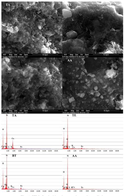
Fig. 6. SEMs for the bituminous rock samples studied.
