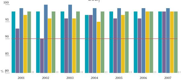
Figure 6.10. Efficiency of wastewater treatment plants over 100,000 population equivalent according to biochemical oxygen demand  $(BOD_7)$ , total phosphorus and total nitrogen in 2001–2007. Data: EEIC.
