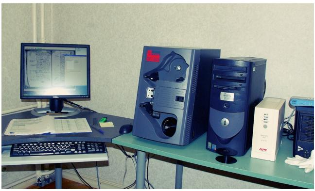
The digitising equipment of Zeutschel microfilms was used to digitise the images of genealogical materials on thousands of microfilms filmed in the 1990s and the first half of 2000s.
