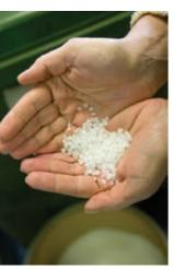
• The mixture is melted at 200 degrees, after which a machine "blows" it into plastic which then needs to be cooled down in order to avoid sticking. Estiko Plastar has the capacity to produce up to 1,500 kilograms of plastic per hour. Its thickness may range from 20 mikrons to 200 mikrons and its width from 20 centimetres to 5.4 metres.
