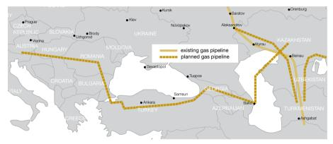
Figure 4. Existing and intended gas pipelines for gas supply from Turkmenistan Source: The Nezavisimaya Gazeta
