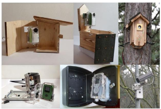
Figure 1: Different boxes to camouflage the cameras (Czachs, C.)
