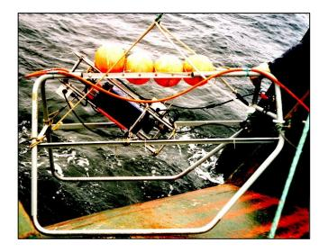
Figure 2.1. The RUV SUBSEA: frame and sledge used in stony (left) and soft (right) bottoms respectively.
