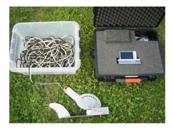
Figure 2.2. Underwater "Drop" camera system operated from small boats. Depth range up to 30 m.
