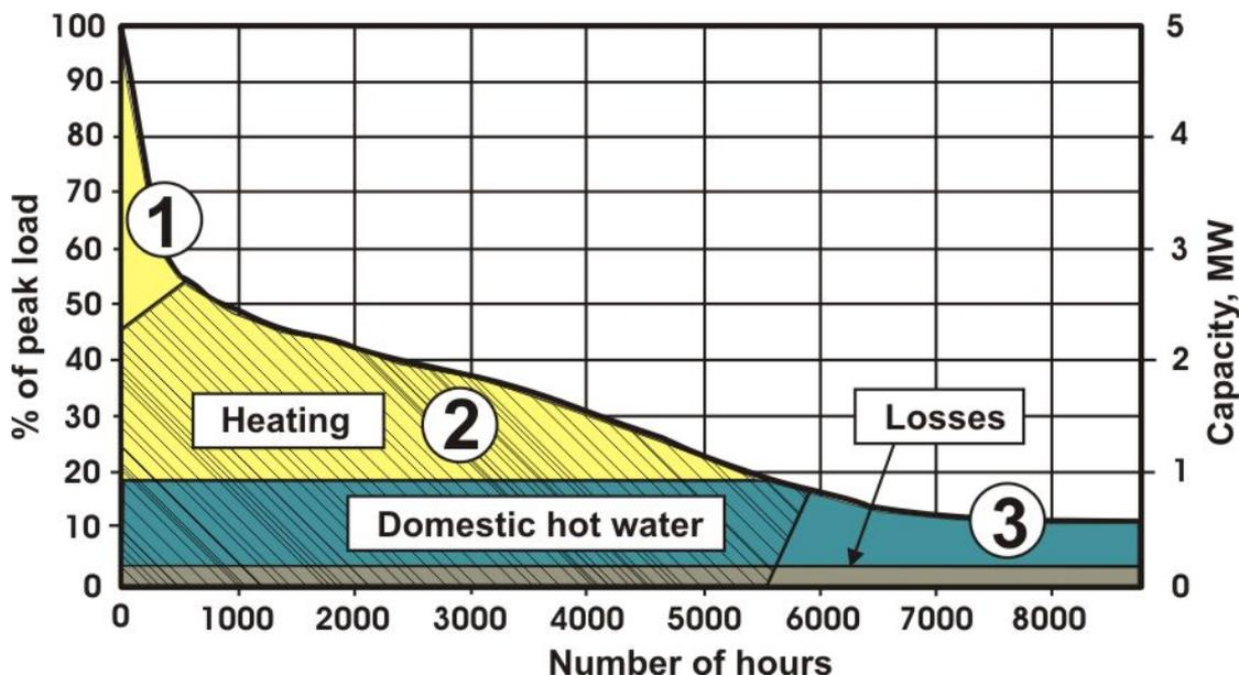
Figure 7.1. Typical load duration curve of DH boiler plant
