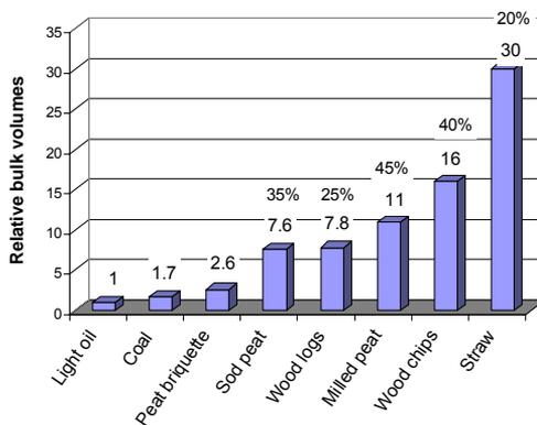
Figure 5.1. Relative bulk volumes of fuel (mean moisture content also shown)
