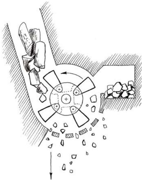
Figure 3.31. A hammer mill
