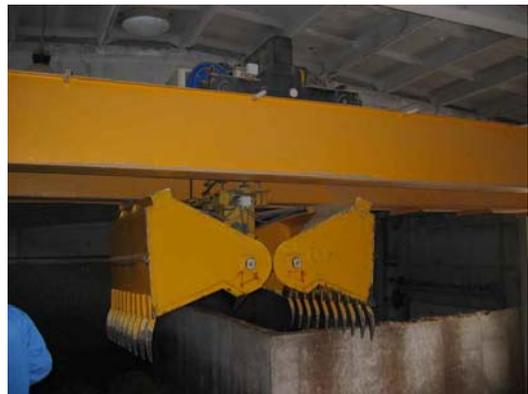
*Figure 8.38. Estonian made bridge crane with grabber, photo by Ü. Kask*
