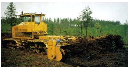
*Figure 3.64. Vegetation stripping and levelling of peat bog surface with the screw leveller RT-6.0H made by the Finnish SUOKONE OY*
