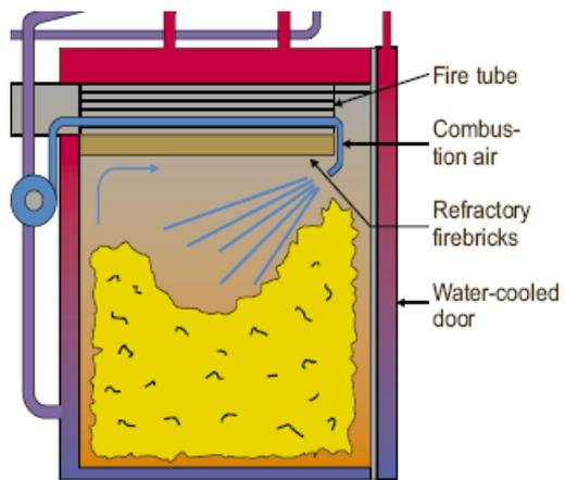
Figure 4.13. The combustion principle of the batch-fired boiler for straw bales [44]
