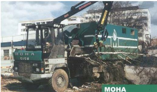
Figure 3.42. The Moha trailer-truck equipped with a chipper [32]
