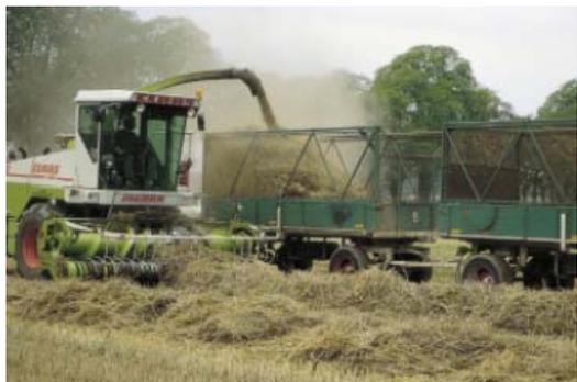
Figure 3.60. A self-propelled chaff cutter in operation [44]
