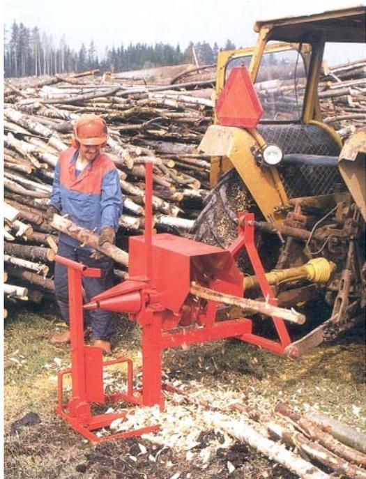
Figure 3.49. Wood chopper combined with a debarker [37]
