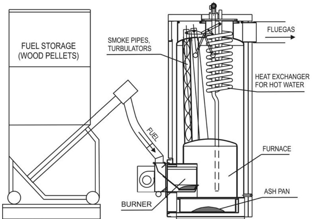
Figure 4.28. The small boiler Pelle with the pellet container, feeder and burner Iwabo VillaS developed at Tallinn University of Technology
