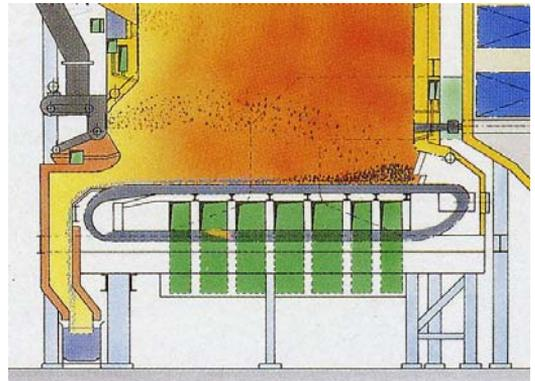
Figure 4.8. Travelling (chain) grate in the boiler of the Borås CHP plant (Sweden)
