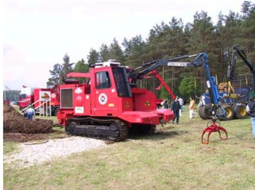
Figure 3.40. An excavator as a base vehicle of chipper, photo by P. Muiste
