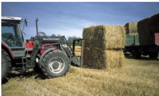
Figure 3.62. Loading of straw bales with a tractor mounted fork lifter [44]
