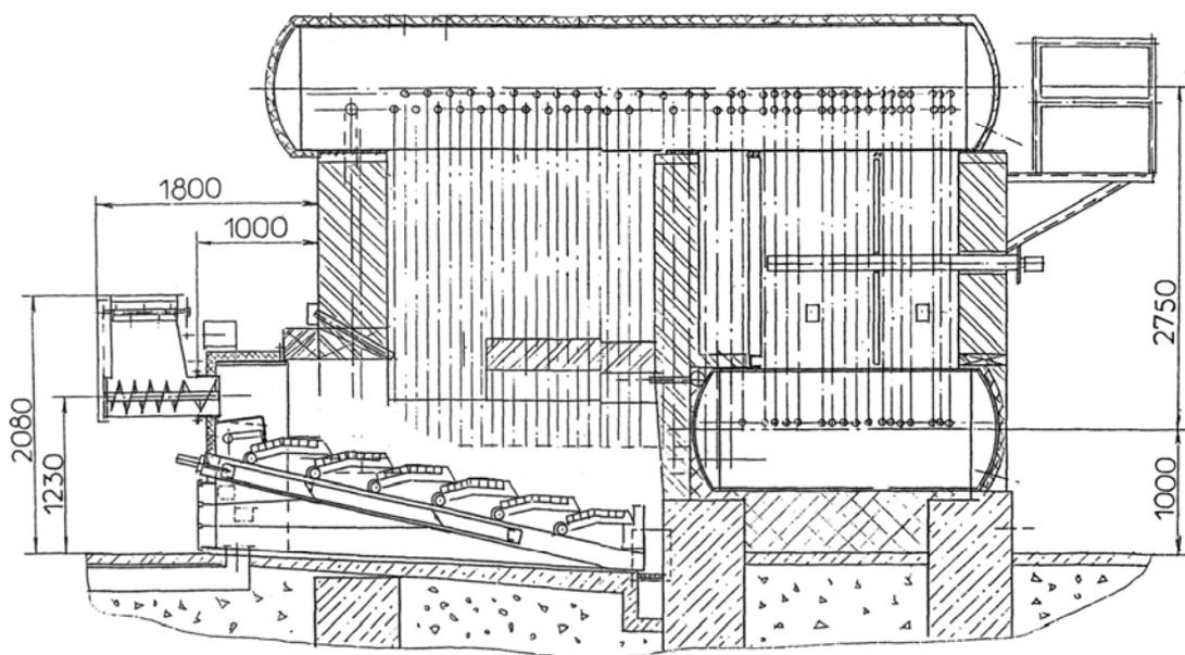
*Figure 8.5. Grate for combustion of woodchips and milled peat installed in the furnace of earlier heavy fuel oil fired DKVR-4-13- type boiler*
