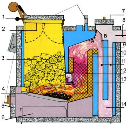
Figure 4.23. The Arimax bottom fired boiler, Högfors Lämpö OY, Finland
