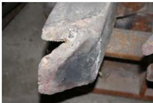
Figure 8.15. A grate bar with the burnt front end, photo by Ü. Kask
