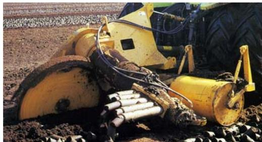
*Figure 3.66. Milling of peat moss from the raised bog surface and extrusion of sod peat with the PK-1S sod cutter of Finnish SUOKONE OY*
