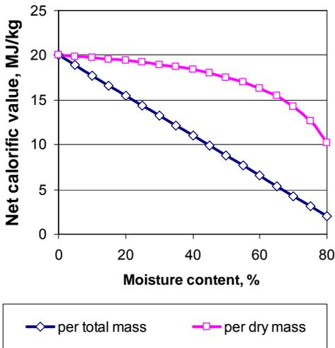
Figure 2.4. Dependence of the net calorific value of wood fuels (as received) on different moisture content
