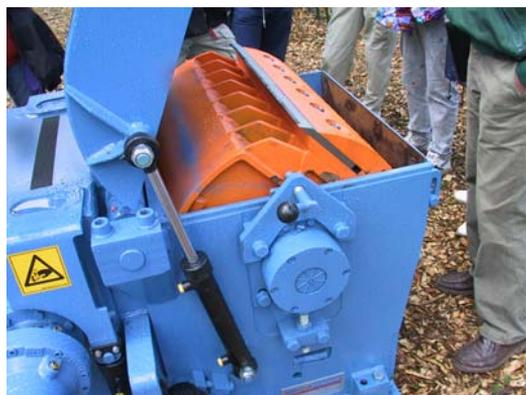
Figure 3.29. The operative part of a drum chipper, photo by P. Muiste
