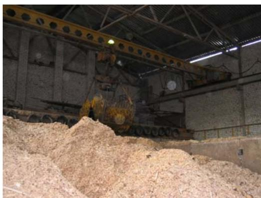
*Figure 8.18. Fuel handling with a grab crane in the fuel storage of Aardla Boiler Plant, photo by Ü. Kask*
