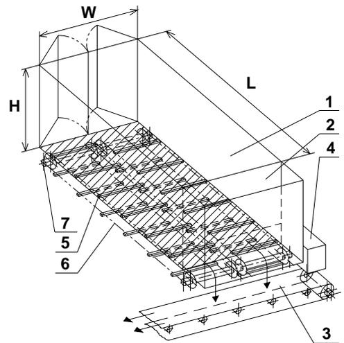
Figure 5.7. Solid fuel bunker with the chain scraper bottom, above photo by Ü. Kask
