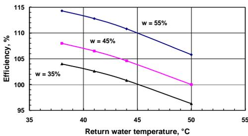
Figure 6.4. Impact of flue gas condensation on the boiler plant efficiency
