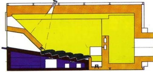
*Figure 4.4. The Swedish Hotab furnace with the grate consisting of fixed and moving inclined parts*
