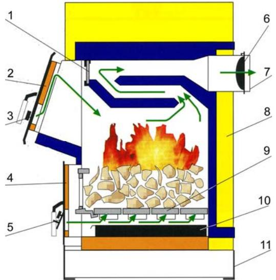
Figure 4.22. A top fired boiler from Eder Ltd (Austria)
