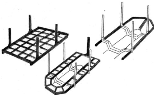
Figure 3.16. Some options for adapting the forwarder for the haulage of logging residues [26]
