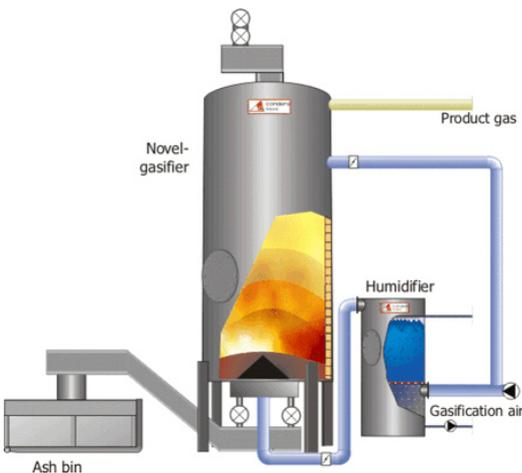
Figure 4.12. The Novel 1–10 MW gasifier of Finnish Condens OY
