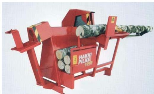
Figure 3.50. The log chopper Hakki Pilke Eagle with a splitting screw and disc saw [38]
