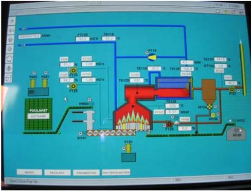
Figure 8.43. Scheme of Peetri Boiler Plant with the operation parameters displayed on the server screen, photo by Ü. Kask
