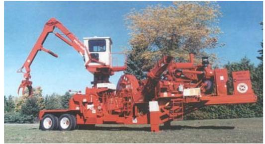
Figure 3.43. The disc chipper Morbark mounted on a trailer 30 [33]
