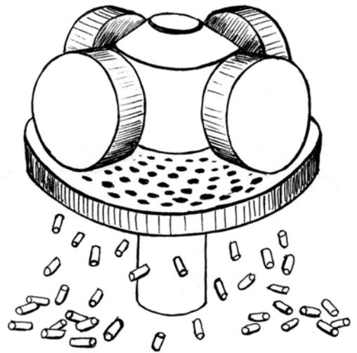
Figure 3.57. Pelletizer with flat die
