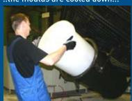
...after a production cycle that typically lasts for one hour, the products can be unloaded from the moulds...
