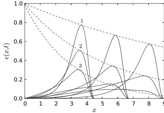
Figure 9: Snapshots of the pulse profiles shown for consecutive time moments, varying the parameter  $\delta$ . The dashed lines show the amplitude decay. For pulse 1 ( $\delta = 0.8$ ) the corresponding amplitude decay function is  $e^{-0.08x}$ ; for pulse 2 ( $\delta = 0.5$ ) the amplitude decay function is  $e^{-0.20x}$ ; for pulse 3 ( $\delta = 0.2$ ) the amplitude decay function is  $e^{-0.32x}$ .
