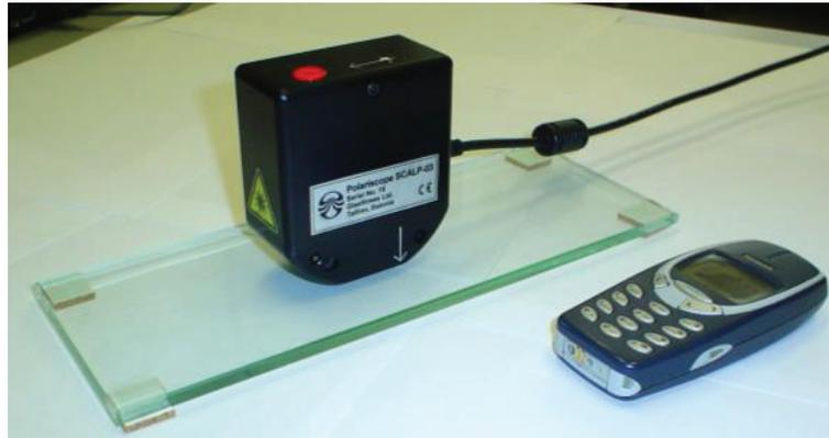
Figure 22: Scattered light polariscope SCALP for stress measurement in architectural glass panels and automotive glazing.
