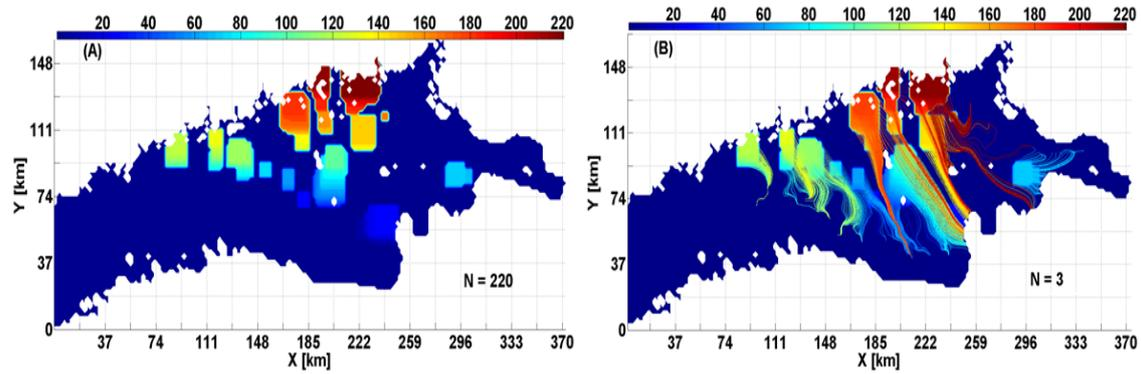
Figure 14: Fow structure in the Gulf of Finland for surface velocity data with a resolution of 1 nautical mile on 17 December 1987 at 18:00. Panels show results for (A) OW method, and (B) hybrid winding-angle method (Viikmäe and Torsvik, 2013).
