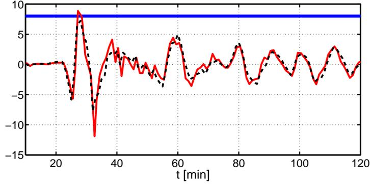
Figure 15: Runup estimates for Samoa 2009 tsunami in Pago Pago made by the assumption of the plane beach (black dotted line) and an inclined bay (red solid line); the thick solid blue line reflects 8 m level of runup measured in Pago Pago (Didenkulova, 2013).
