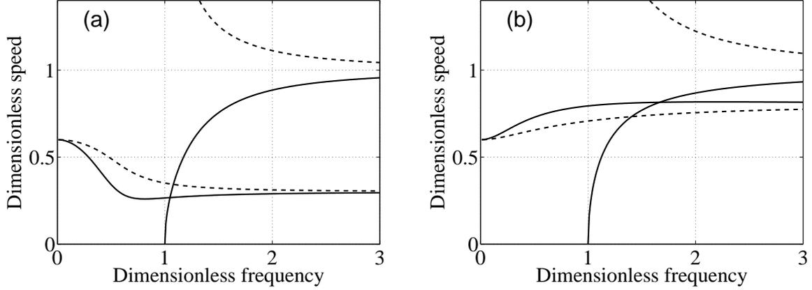
Figure 2: Group (solid line) and phase (dashed line) speed curves for (a) normal dispersion case and (b) for anomalous dispersion case.
