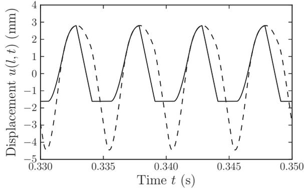
Figure 8: Four periods of the string displacement for the nonlinear bridge with a small geometric imperfection are shown by solid line. The corresponding linear case is shown by dashed line.
