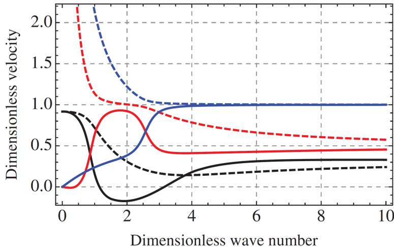
Figure 3: Blue - upper optical dispersion branch, red - lower optical dispersion branch, black - the acoustical dispersion branch. Phase (dashed lines) and group velocity (solid lines) curves against wave number for the Mindlin-type model at material parameter combination resulting in NGV
