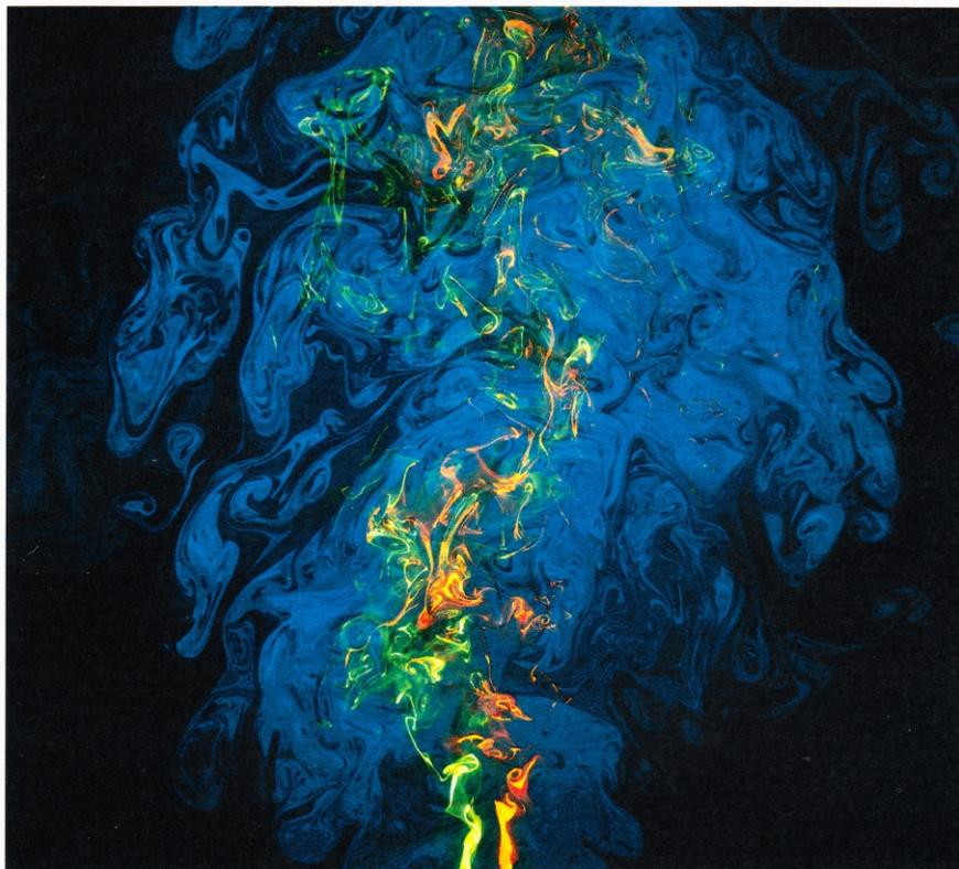
Fig. 1. from the paper by *M.Kree et al.* **The mixing of distant sources.** The image shows a two-dimensional cut through the instantaneous concentration fields  $c_1$  and  $c_2$ .
