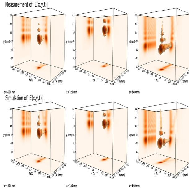
Figure 28: Measured (top) and simulated (bottom) impulse response of type IV Airy pulse generator consisting of a custom-made continuous cubic phase element and a Fourier lens  $f = 500\text{mm}$  at three propagation distances. Color represents the relative amplitude of the electric field isosurfaces. The images show projections of the pulse to the corresponding planes.
