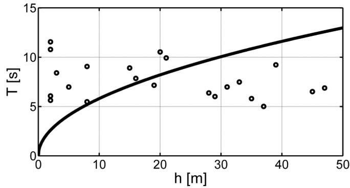
Figure 17: Rogue wave period plotted against the water depth of their occurrence; black solid line corresponds to the criterion of the modulational instability.
