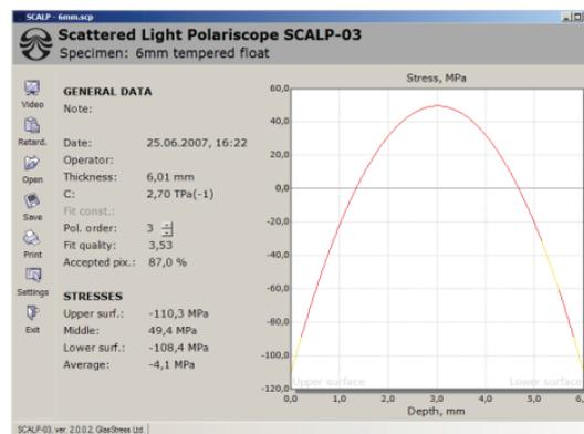
Figure 23: Stress profile through the thickness of an architectural panel.
