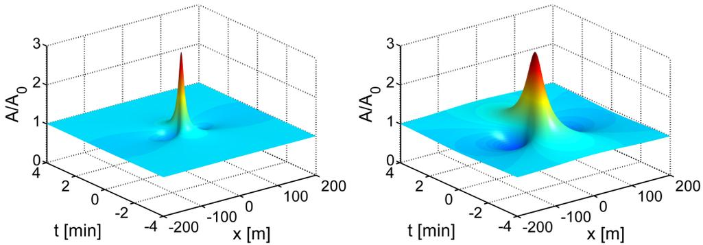
Figure 18: The Peregrine breather at the background of the carrier wave with the period 6 s and amplitude  $A_0 = 3$  m for (a)  $kh = \dots$ ; (b)  $kh = 1.6$  (Didenkulova, Nikolkina et al., 2013).
