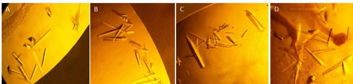
**Figure 13. Crystallization of LMCA1 double mutant.** Crystals of LMCA1 double mutant are represented in this figure. Crystals appeared in the condition containing 18% PEG6000, 12% glycerol, 3% t-BuOH, 140 mM  $\text{MnCl}_2$ , 5 mM  $\beta\text{ME}$  and second detergent: A. 144 mM sodium dodecanoyl sarcosine (sarcosyl), B. 32 mM n-Nonyl- $\beta$ -D-thiomaltoside, C. 4 mM ZWITTERGENT 3-14, D. 43 mM DDMAB.
