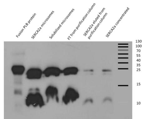
**Figure 16. Detection of PLB in SERCA2a samples.** Fusion PLB was used as a positive control, the expected mass is 35kDa. In all fractions (microsomes, solubilized microsomes, FT from purification column, and in the eluted and concentrated protein fractions) PLB has been detected. PLB monomer can be seen at 11 kDa, the bands at 25 kDa are considered PLB pentamers.
