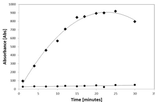
**Figure 11. The activity of LMCA1 triple mutant (M59L, S240G, S295P).** The activity of constructed LMCA1 triple mutant was tested using Baginski assay. LMCA1 WT is represented in rhombs, LMCA1 triple mutant in circles. No inorganic phosphate was released after 30' of incubation time.
