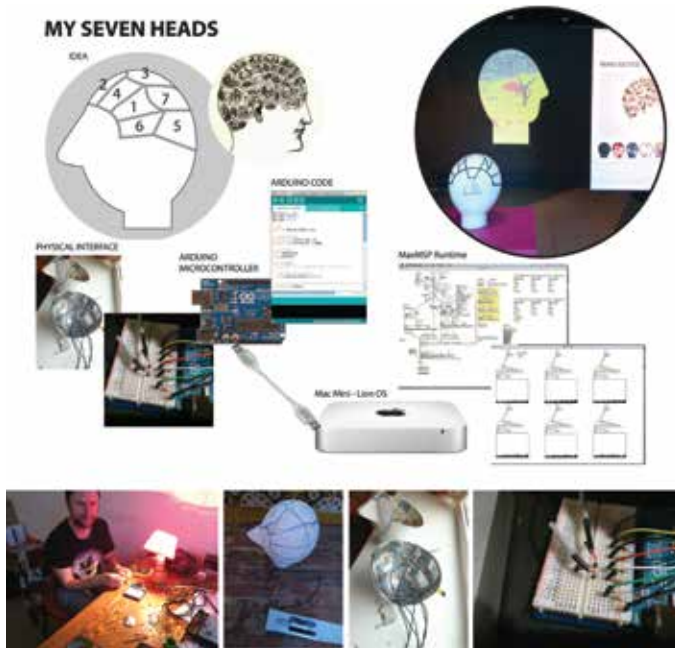
Figures 12: Technological structure of installation and archive photos (2012–2013)
