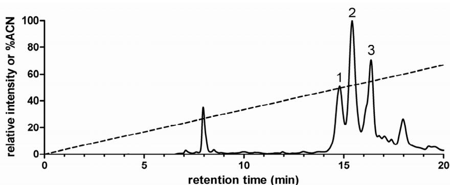
**Figure 9.** The monitoring of the removal of protecting groups by RP-HPLC. The final product Adc-Ahx-(L-Arg)<sub>4</sub>-L-Lys-NH-PEG5000-OMe (ARC-701; **1**, R<sub>t</sub>=14.8 min) and intermediate products bearing one (**2**, R<sub>t</sub>=15.4 min) or two (**3**, R<sub>t</sub>=16.4 min) Pbf groups. The dashed line represents linear water-ACN gradient (0–100% ACN/30 min; 0.1% TFA; 1 ml/min).
