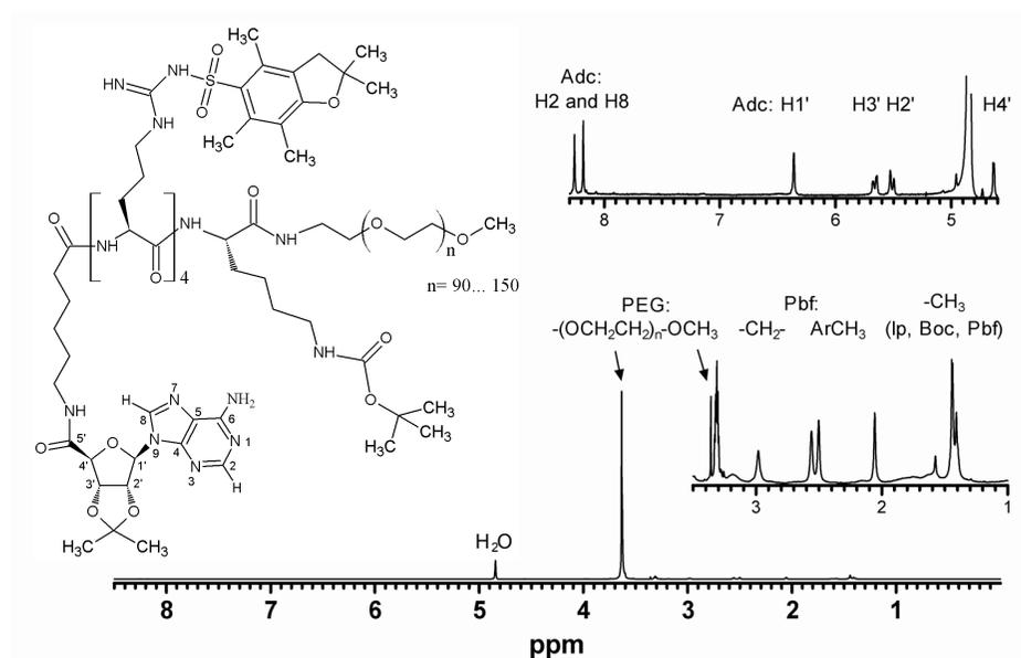
**Figure 7.** The structure and <sup>1</sup>H NMR spectrum (200 MHz) of ARC-701 bearing protecting groups, Adc(Ip)-Ahx-[L-Arg(Pbf)]<sub>4</sub>-L-Lys(Boc)-NH-PEG5000-OMe (75 mg/ml in CD<sub>3</sub>OD). Magnifications are given as insets.
